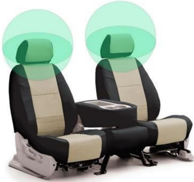
The **Quiet Bubble™** was already installed on a vehicle and proved to be efficient in low-medium frequency noise reduction. The system offering an appealing dB/Kg ratio, when applied instead of passive NVH solution. The **Quiet Bubble™** can also be used in addition to the passive means for creating "super quiet" environment.
